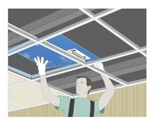
Then set the light box on top the Elevator/SkyTile sandwich.
