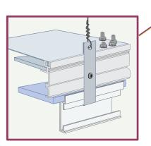
Insert the assembled fixture into the grid much as you would a ceiling tile.
