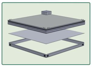
Use the hanger brackets to secure the Elevator to the light box.
