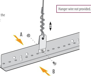
**Note:** Where possible, do not hang adjacent runners in the same 2' x 2', 60cm x 60cm, or 62.5cm x 62.5cm opening: installation of the fixtures may require one open side above the grid into which they can be temporarily inserted before dropping down into the grid pocket.
